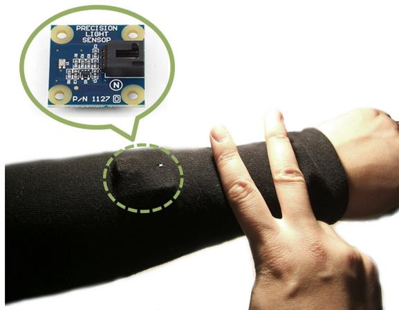
Figure 6: Touch scanner prototype based on a Phidgets light sensor board connected to a PC. To simulate the notion of a disappearing mobile device, we hide the device under the sleeve of a sweatshirt; a 1mm hole exposes the sensor.
