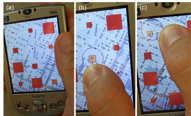
Figure 1. (a) Small targets are occluded by a user's finger. (b) The proposed *Shift* technique reveals occluded screen content in a callout displayed above the finger. This allows users to fine tune with take-off selection. (c) By adjusting the relative callout location, Shift handles targets anywhere on the screen.
