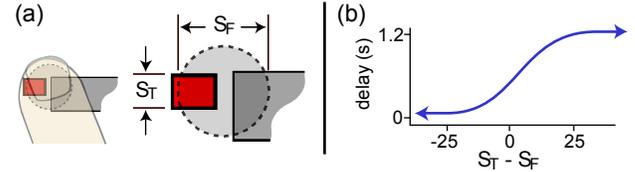
**Figure 8. Ambiguity estimation for escalation:** (a) the occlusion threshold diameter  $S_F$  and the smallest dimension of the smallest target found under the finger  $S_T$ ; (b) logistic function maps the difference  $S_T - S_F$  to a dwell timeout.
