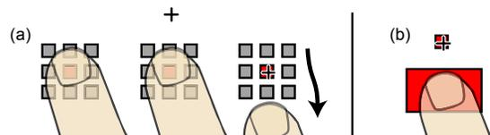
**Figure 3. Shift’s conditional escalation is not practical for Offset Cursor:** (a) escalating to an Offset Cursor requires a large corrective movement; (b) users might avoid this by aiming below the target, but then default escalation may be ambiguous. Is the user trying to select the large target or waiting for an offset pointer to appear to help acquire the small target?
