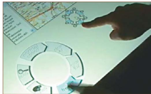
**Figure 3. Dual-finger selection on multitouch tabletop display.** The user manipulates the pointer with the right hand while adjusting the control-display ratio with the left.
