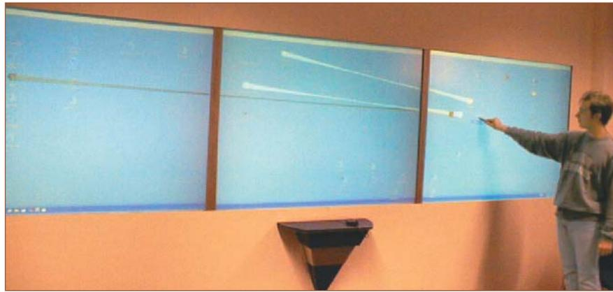
**Figure 2. Drag-and-pop technique.** As the user drags an icon from the right panel to the center, potential target folders "stretch" toward him, enabling him to file the icon with a small hand movement.
